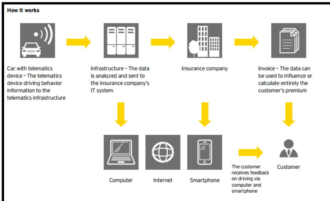
Fig. 2. The information flow of Usage Based Insurance (EY. (2016). *Introducing "Pay How You Drive" (PHYD) Insurance.*)
