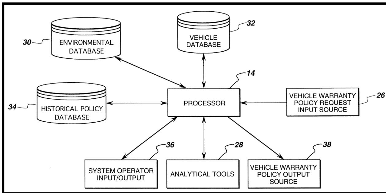
Fig. 3. The processing architecture of the automated risk-based pricing system (Osborn, B. E., & Hershey, J. E. (2001). (12) United States Patent.
